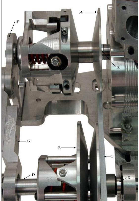
To properly align your Shockwave front clutch and 7" reverse driven for operation you will need the following items:
